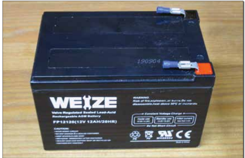
A small 12-volt, 10-amp-hour battery. This one is what I use to keep the hangar radio going using the small 1.5-watt (100 mA) charger on a constant float charge.
