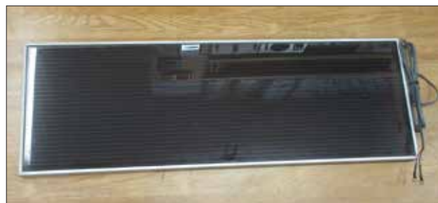
This 25-watt solar panel (left) produces about 2 amps output in full sunlight or a bit less on a cold winter day in moderate sunlight. This small 1.5-watt solar panel (right) used to keep the 10-amp-hour radio battery on continuous charge.
